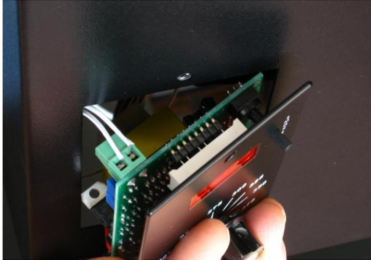
**WARNING: Do not force the control into the cutout. Bumping electronic components into the edge of the cutout during installation may damage the control.**
